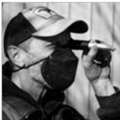
Tom Janda checking sugar concentration with a Refractometer
